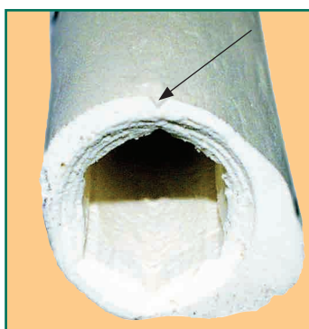
Fig. 1: Hexagonal implant bed in a bone model
