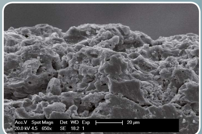
detailed view of implaFiX® HA coating (200x increase)
