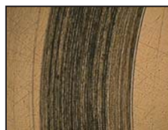
Surfaces after Pin-on-Disc-Test with bone cement, TiN (left), non-coated titanium (right)
