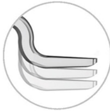
3 different hook depths 12, 15 and 18 mm
